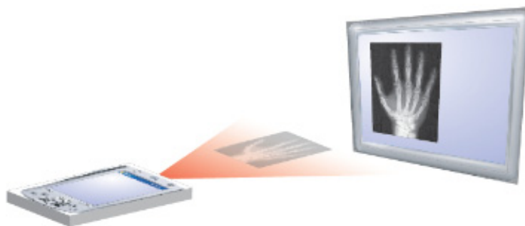
Figure 58: A mental model where the image is sent by IR to the patient terminal from the PDA.
