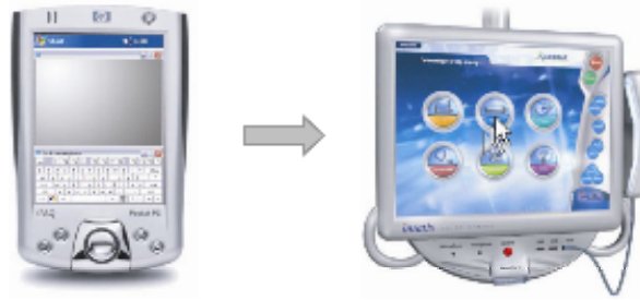
Figure 29: The PDA offers a touch pad and a virtual keyboard to control the patient terminal
