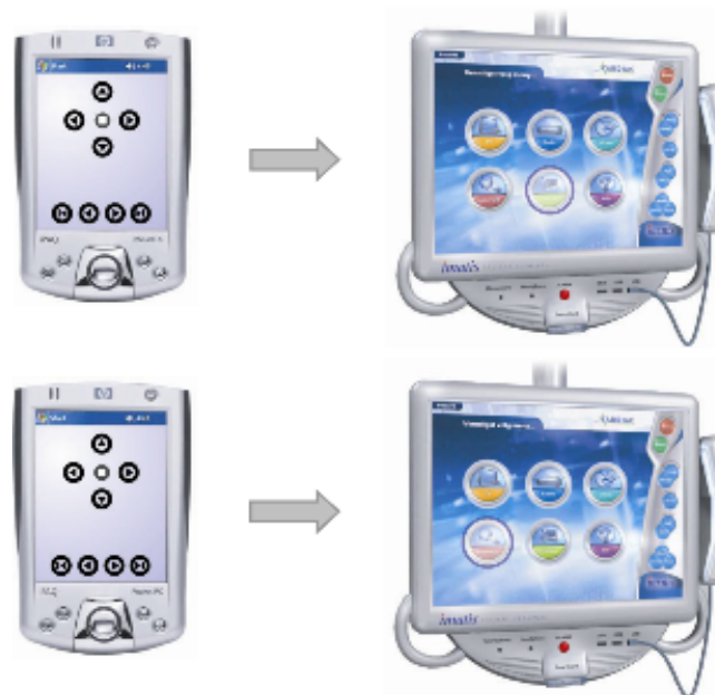
Figure 28: The PDA is a remote control that can be used to navigate through choices and menus. A click on the left arrow will cause the highlighted button to change
