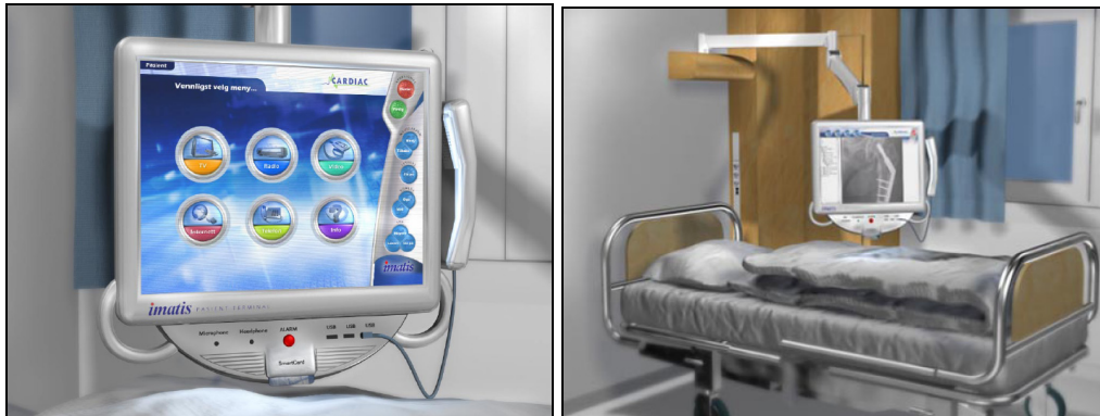
Figure 22: The patient terminal offers patient-centered services and is mounted on a movable arm (Illustrations from Cardiac AS)
