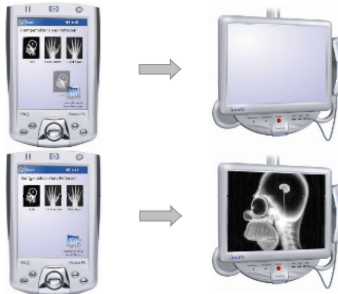
Figure 30: The PDA displays information objects, here as x-ray images. Objects can be dragged and released over an icon representing the patient terminal. The information object is then transferred from the PDA to the patient terminal
