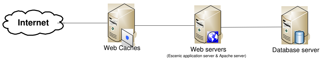
Figure 3.4: Major components in the TV2i system
