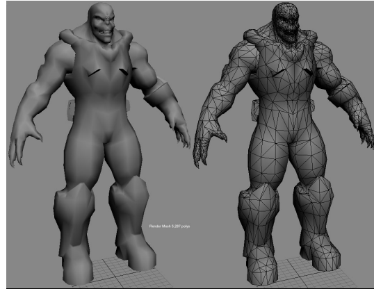
Figure 2.10: 5,287 triangle in-game mesh in 3D Studio Max. [Tec04]
