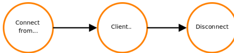
Figure 9.4: Illustration of the normal flow of messages from postfix/smtpd in the example log file found in Appendix A.3
