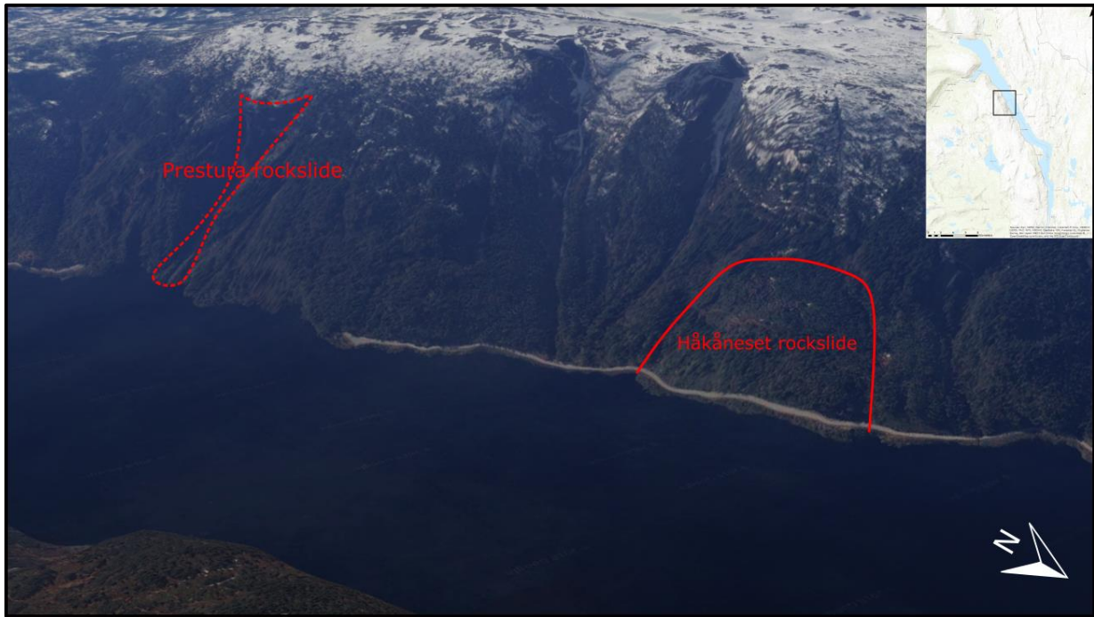
Figure 5: 3D image of the unstable Håkåneset rockslide to the right and the prehistoric Prestura rockslide to the left. Located at the western margin of lake Tinnsjø. The outline of Håkåneset is defined by Sollie (2014), based on old bathymetrical data. Modified from Google earth.
