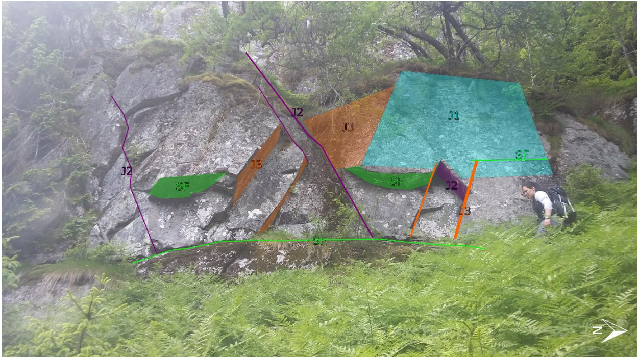
Figure 41: Locality C4 (see appendix E) north of the release surface. J1, J2, J3 and SF is evident in the terrain. J2 and J3 is creating small wedge failures along the steepest slopes. While SF is cutting J1 dipping into the slope.
