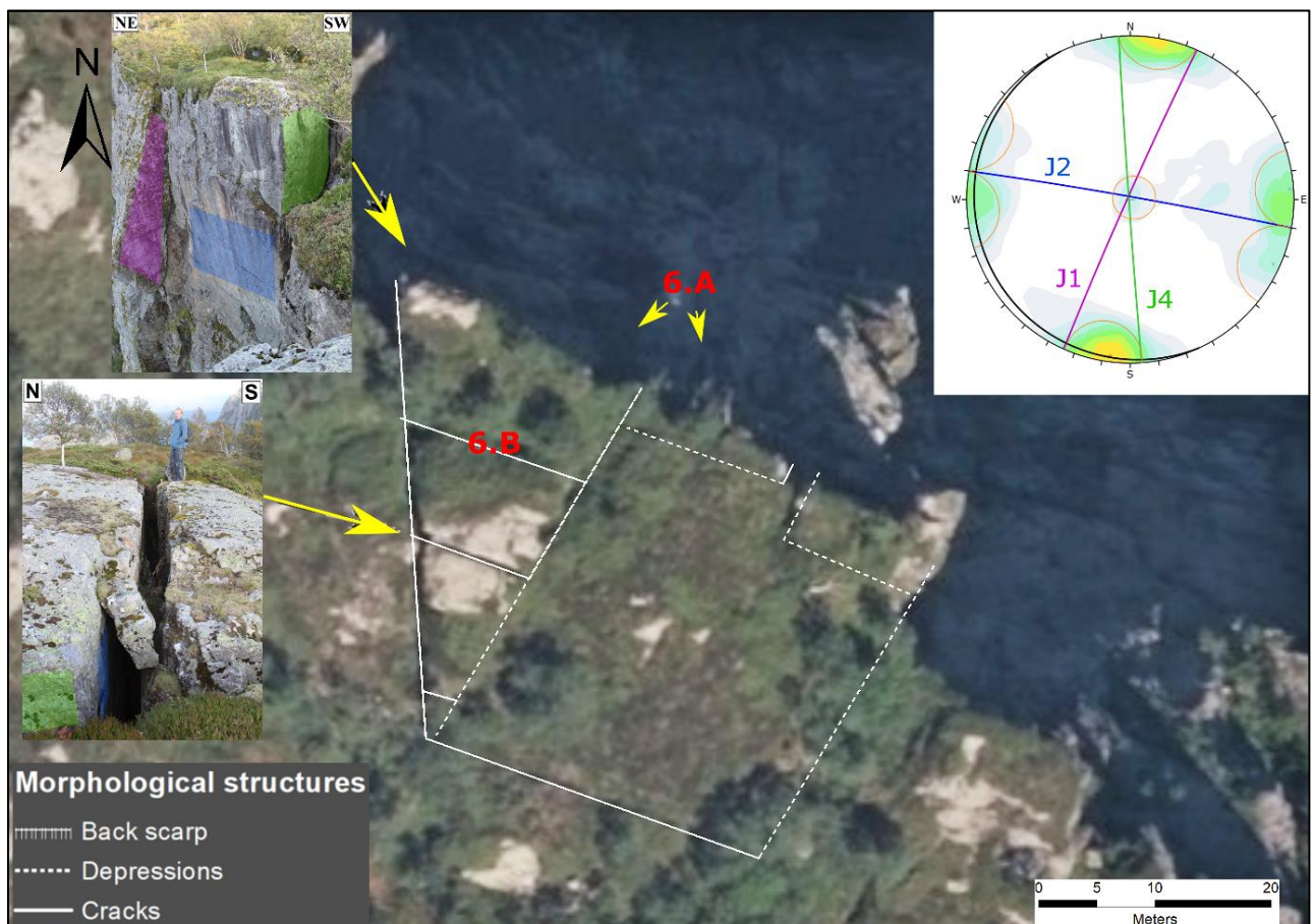
Figure 4.27: Orthophoto of location 6 with drawn morphological structures detected in the field. Pictures are showing delimiting structures, both back scarps following the orientation of J2 and flanks following the orientation of J1 and J4. The stereonet shows that the structures at the orthophoto coincide with the significant structures of the mid domain.
