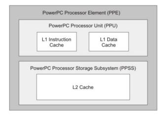
Figure 2.2: The architecture of the PPE. Taken from [24].
