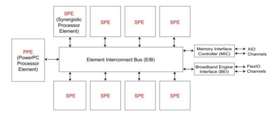
Figure 2.1: The Cell/BE architecture. Taken from [24].
