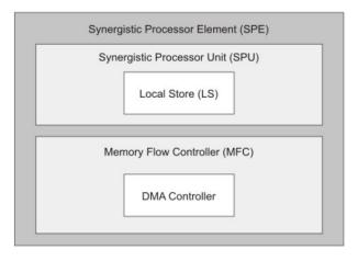
Figure 2.3: The architecture of an SPE. Taken from [24].
