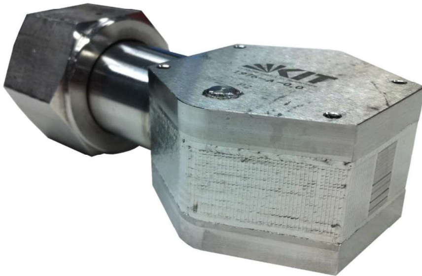
Figure 3: Photo of the microstructured body (MSB) used in hot-wire anemometry measurements.
