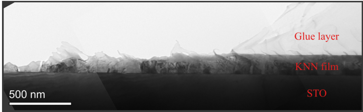
Figure 4.3: BF image of specimen P450S-II obtained in TEM. The image is a combination of three separate BF images.
