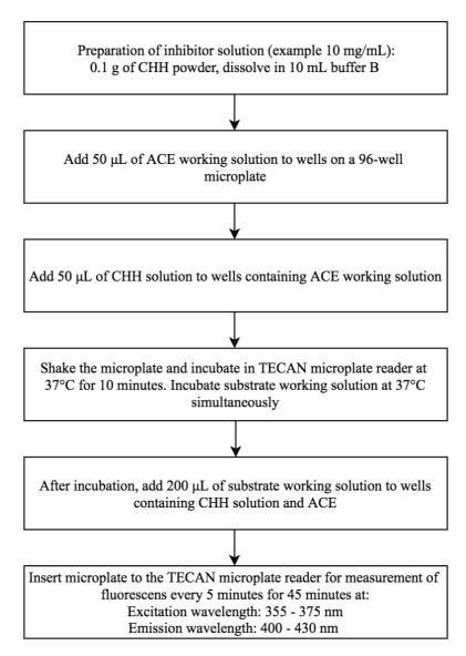
**Figure 2.4:** Flowchart describing the experimental procedure for measuring the ACE inhibitory activity of CHHs (Sentandreu and Toldrá, 2006).
