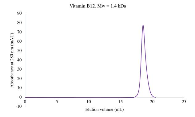
**Figure D.4**: Chromatogram from gel filtration of vitamin B12 analyzed by FPLC using the column Superdex Peptide 30/100 GL. Vitamin B12 has molecular weight 1 356 Da, and the peak was detected at elution volume 18.54 mL.
