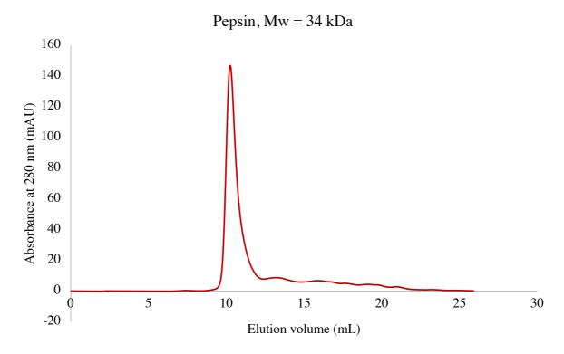
**Figure D.1:** Chromatogram from gel filtration of pepsin analyzed by using FPLC and the column Superdex Peptide 30/100 GL. Pepsin has molecular weight 34 000 Da, and the peak was detected at elution volume 10.29 mL.
