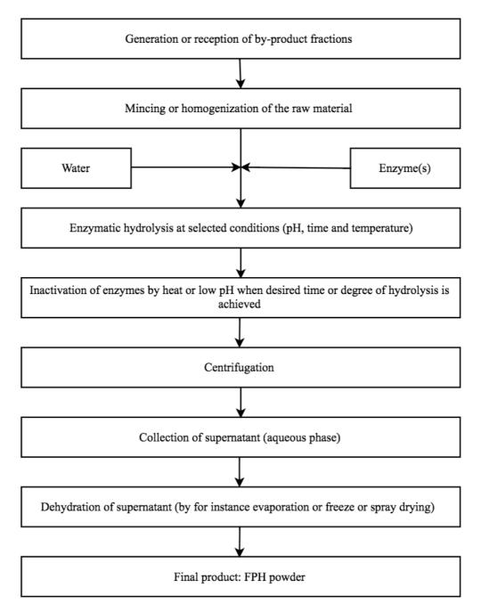
**Figure 1.2:** Flowchart describing the general steps in an enzymatic hydrolysis for production of FPH from marine by-products. The figure is modified from Kristinsson and Rasco (2000b) and Benjakul *et al.* (2014).
