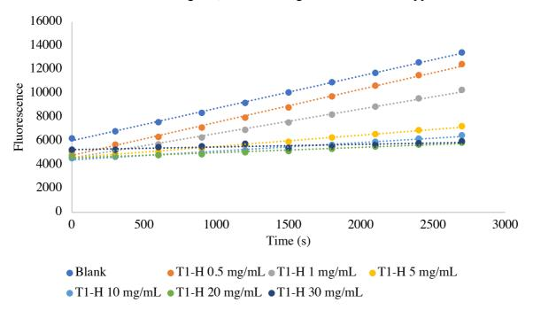
**Figure B.1:** Fluorescence plotted against time (seconds) for concentrations of hydrolysate T1-H investigated for ACE inhibitory activity. The negative control is denoted "blank".
