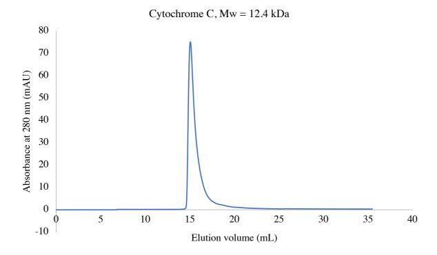
**Figure D.2:** Chromatogram from gel filtration of cytochrome C analyzed by FPLC using the column Superdex Peptide 30/100 GL. Cytochrome C has molecular weight 12 384 Da, and the peak was detected at elution volume 15.1 mL.
