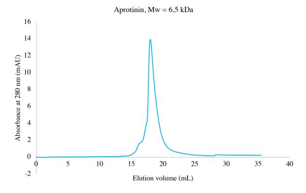
**Figure D.3**: Chromatogram from gel filtration of aprotinin analyzed by FPLC using the column Superdex Peptide 30/100 GL. Aprotinin has molecular weight 6 512 Da, and the peak was detected at elution volume 18.0 mL.
