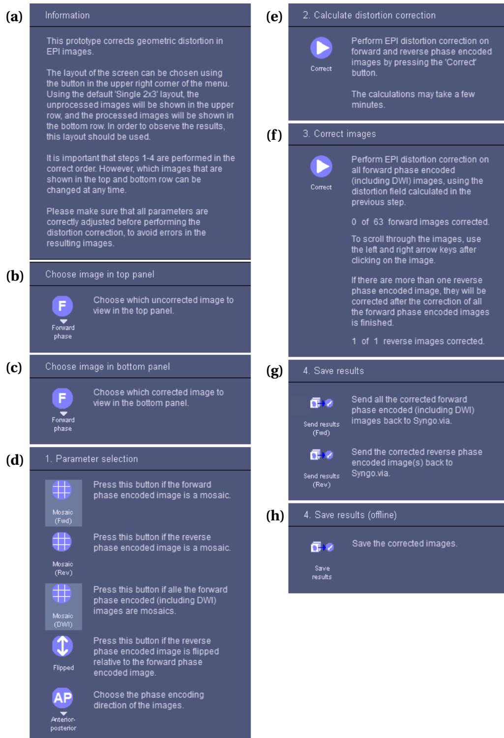
Figure 4.4: Tabs of the sidebar menu. (a) Information to the user about how to perform the distortion correction. (b) , (c) Let the user select which uncorrected and corrected image to be rendered in the top and bottom row of the screen, respectively. (d) Parameters that the user can select for the distortion correction. (e) The user can calculate the distortion correction from the forward and reverse phase encoded b_0 images. (f) The user can correct the other images. (g) The user can send the results back to the syngo.via server. (h) Additional step for saving the corrected images locally when testing the prototype (this step is not included in the final, installed version of the prototype).
