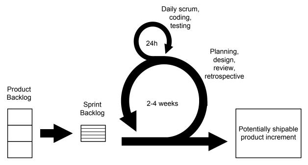
Figure 2: Cycles in the Scrum methodology (Schwaber, 2004, p. 6)
