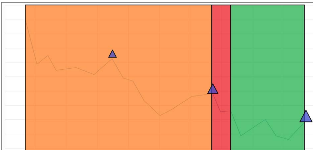
Figure 10: Illustration of different opinions of identification. Blue triangles represent what the author would identify as steps. Coloured sections represent step-pool sequences identified by the algorithm.
