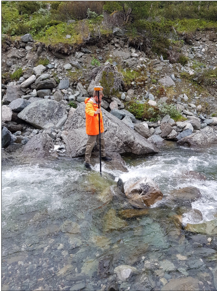
Figure 7: Measuring the bed with GNSS point measuring. The operator on land would set the point when the measuring rod was securely placed.
