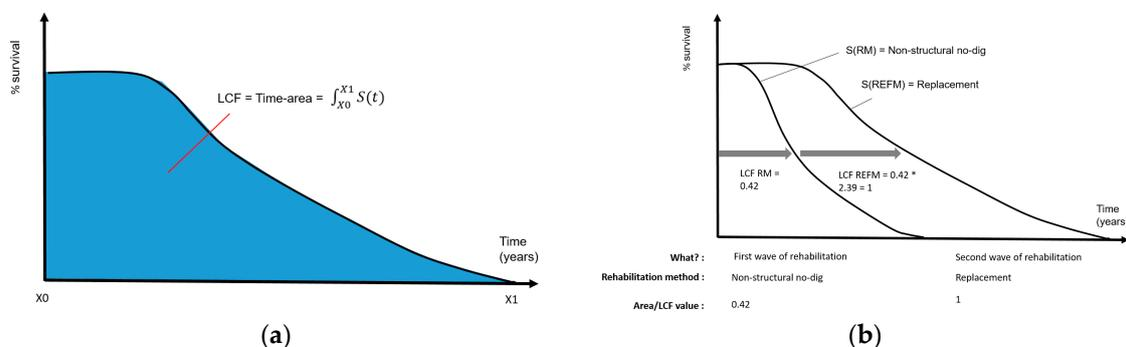
**Figure 3.** (a) Illustration of the time-area idea which is the concept the LCF is built upon. (b) Illustration of the correlation between LCF and SF values for non-structural no-dig and the reference method (replacement).
