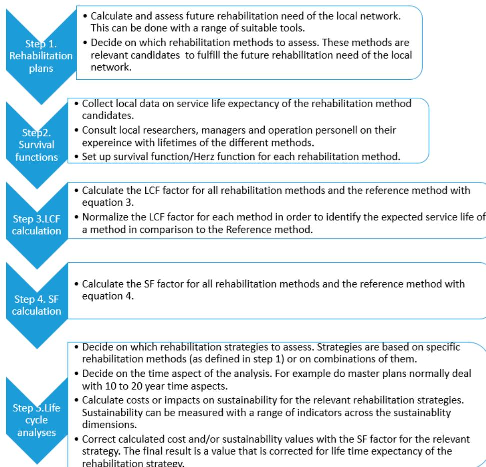
**Figure 2.** A flow chart of the process to create and use SF-factors in long-term planning and management of urban water networks.
