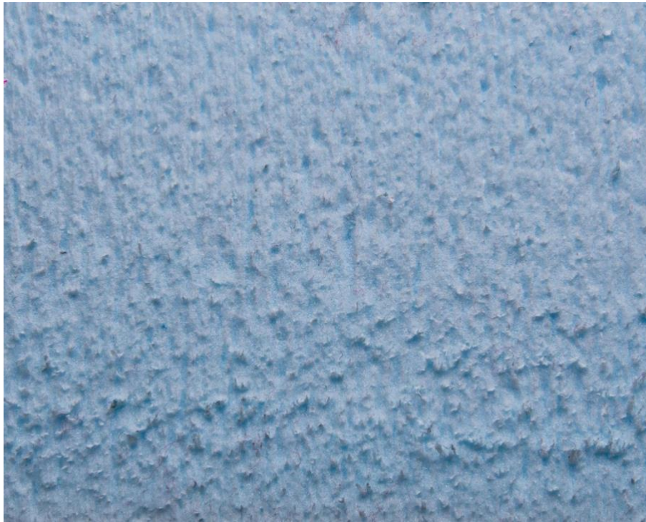
Figure 3: Close-up photo of XPS cut surface. Photo: Sigurd Vaagland
