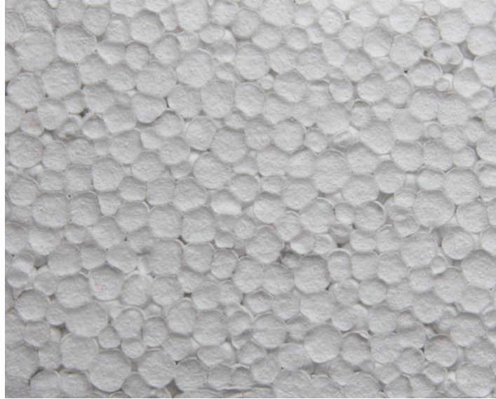
Figure 2: Close-up photo of EPS cut surface. Photo: Sigurd Vaagland
