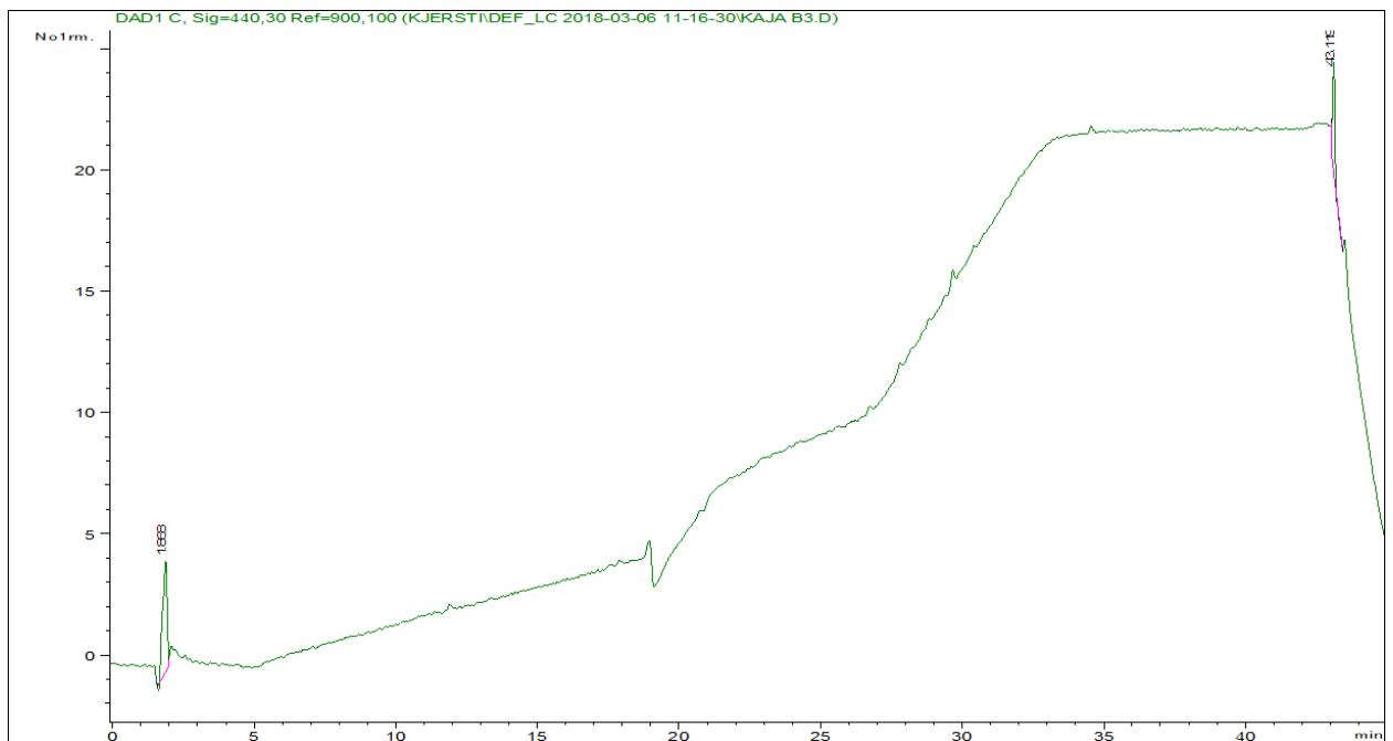
Figure 0.1: Results of the High Performance Liquid Chromatography (HPLC) analysis conducted to identify phytoplankton pigments from the sediment samples from the study site 6 km south of the mouth of the Trondheimsfjord, Norway. The x axis shows time in minutes and the y axis shows area at 440 nm absorbance. The results show no peaks hence indicating no presence of phytoplankton pigment in the sample. The result of this sample is representative for all samples conducted.
