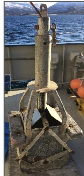
Figure 2.5: Box core with 30x30 cm area and a volume of 0.117cm 3 for sediment samples the 22nd of February 2017. Photo: Kaja Lønne Fjærtøft.
