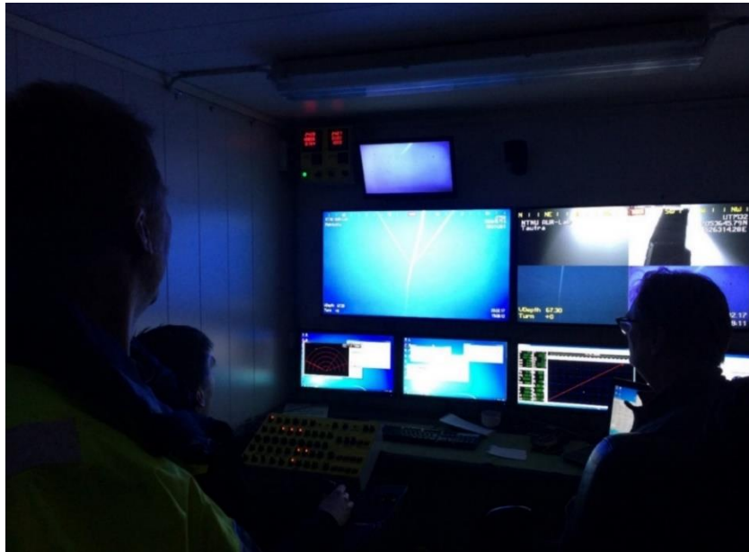
Figure 2.4: The control room for the Remotely Operated Vehicle (ROV), with the joystick on the bottom left. The screen displays live footage from the ROV transmitted by optical fibres to the surface via the umbilical, and biological objects of interest and habitat types can be live logged with exact location utilising the software Urd. Photo: Kaja Lønne Fjærtøft
