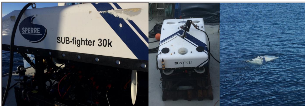
Figure 2.3: The Remotely Operated Vehicle used for the transects was a Sperre SUB-fighter 30k equipped with halogen lights, HMI gas lights and a high-resolution video camera with a laser ruler (distance=10cm) to enable a scale for the images. Photos: Kaja Lønne Fjærtøft.
