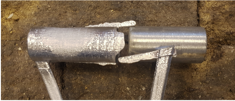
Figure 5.3: Image of a casting with blunt steel insert which broke upon mold removal.
