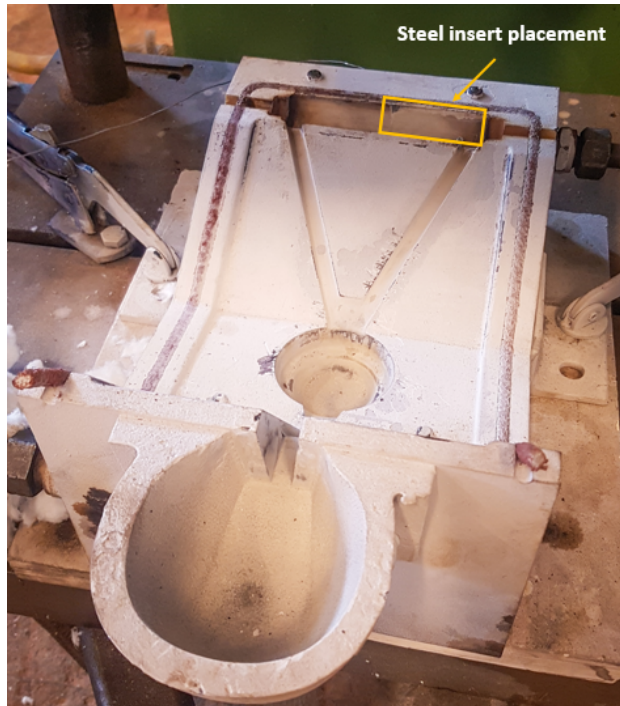
Figure 5.2: Casting mold used in lab scale shape casting experiment. The yellow area indicates placement of the steel inserts.
