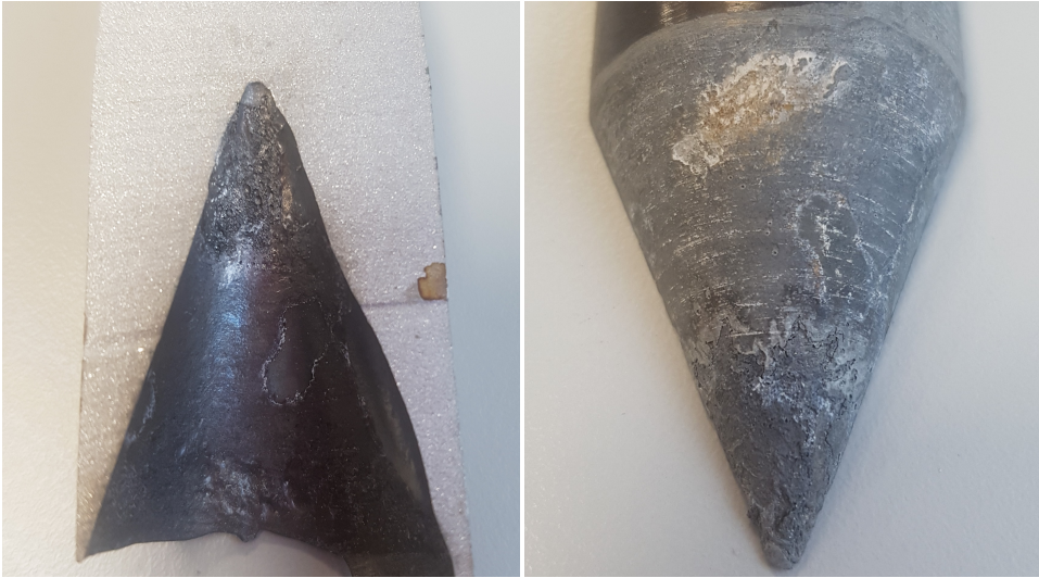
Figure 5.16: Image of cast aluminum and steel insert, from left to right respectively, for Casting N after tempering and breakage.
