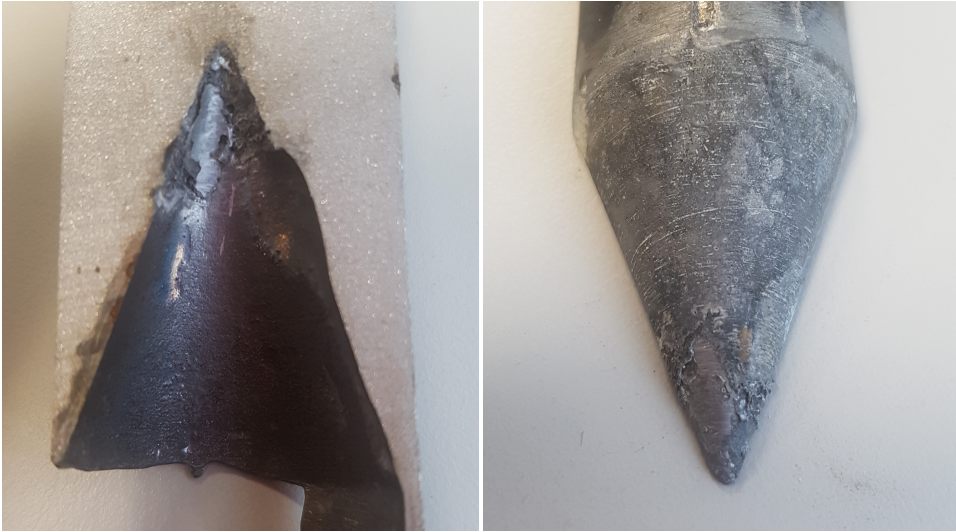
Figure 5.17: Image of cast aluminum and steel insert, from left to right respectively, for Casting O after tempering and breakage.
