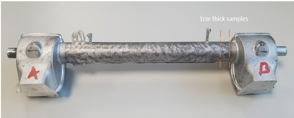
Figure 3.2: Cutting pattern for low pressure die casting samples.
