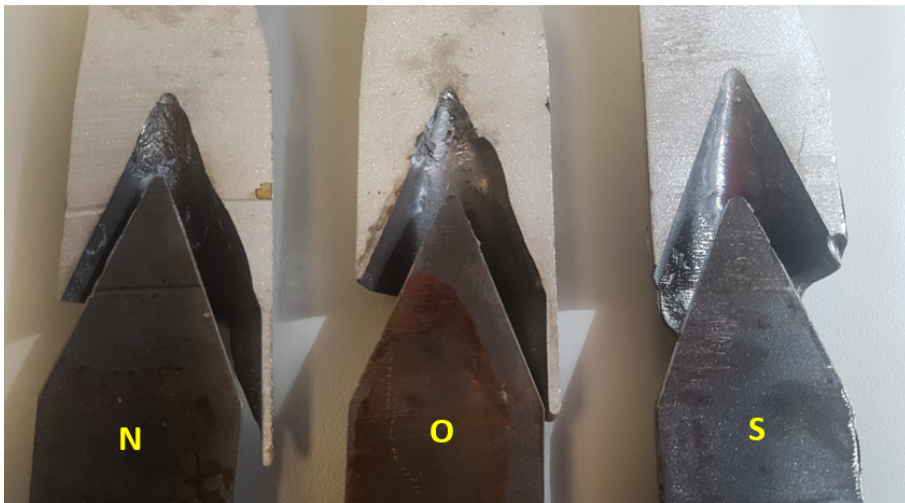
Figure 5.15: Image of Casting N, O and S after tempering. In all castings, the steel insert loosened from the cast aluminum.
