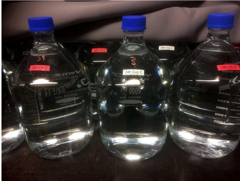
Figure 5: Naphthenic crude oil WAF exposure. 20 bottles were filled with filtered seawater for the control groups and 16 with the WAF medium for the exposed groups. Bottles were kept at 10 °C and covered with a dark blanket to avoid light interference with the medium.
