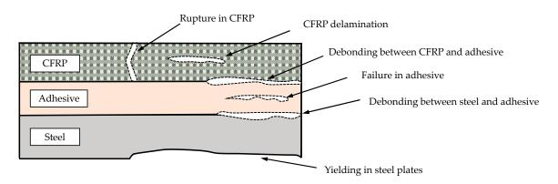
Figure 12. Different types of failure mechanisms in steel/CFRP bonded joint.
