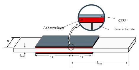
Figure 1. A schematic of steel/CFRP double strap joint.
