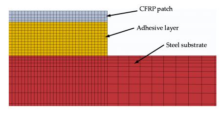
Figure 5. A typical mesh pattern used for DSJ models.
