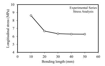
**Figure 8.** The variation of critical longitudinal stress for different bonding lengths (applied stress for all the specimens: 1000 MPa).
