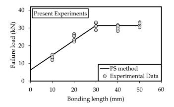
Figure 9. Comparison between the experimental failure loads of DSJs and the theoretical predictions obtained by means of point stress (PS) method.
