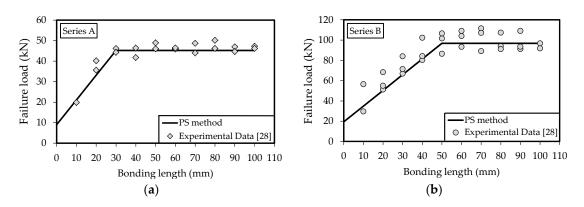
**Figure 11.** Comparison between the experimental failure loads of DSJs and the theoretical predictions obtained by means of PS method; (**a**) series A; (**b**) series B.
