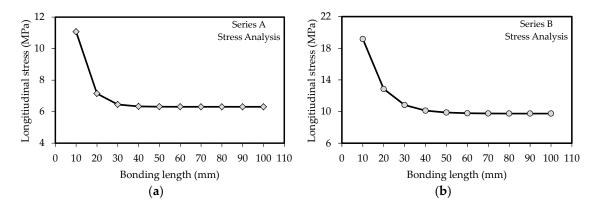
**Figure 10.** The variation of critical longitudinal stress for different bonding lengths (applied stress for all the specimens: 1000 MPa); (**a**) series A; (**b**) series B.
