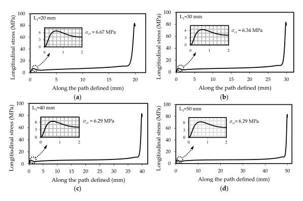
**Figure 7.** Longitudinal stress distribution along the path defined in the mid-plane of the adhesive layer for the present experimental series—(a)  $L_1 = 20$  mm; (b)  $L_1 = 30$  mm; (c)  $L_1 = 40$  mm; (d)  $L_1 = 50$  mm (applied stress for all the specimens: 1000 MPa).
