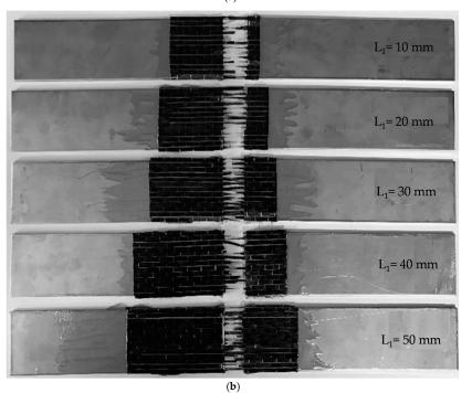
Figure 2. Double strap joints (DSJs) prepared for experiments (a) before the test; (b) after the test.
