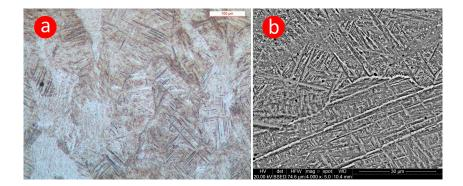
**Figure 5.** Optical Microscope (**a**) and Environmental Scanning Electron Microscope (**b**) micrographs of the analyzed material.
