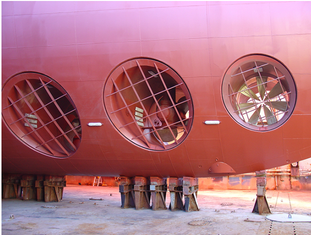
Figure 3: Illustration photo of a tunnel thruster, courtesy of Brunvoll AS
