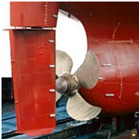
Figure 1: Illustration photo of a main propeller with rudder, courtesy of Becker Marine Systems and Kongsberg Maritime
