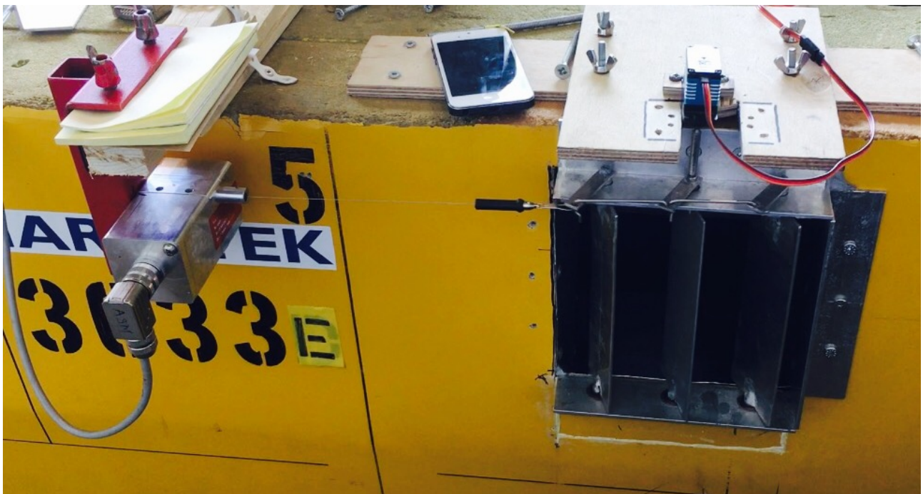
Figure 5.11: Servo test setup with pull cord displacement sensor.
