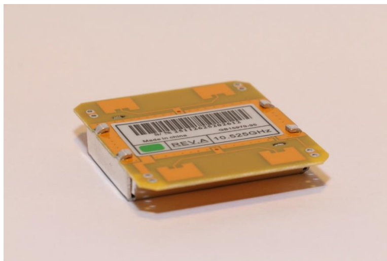
Figure 4-8 HB100 MC420S back side with PCB-antennae patches visible as four small squares.
