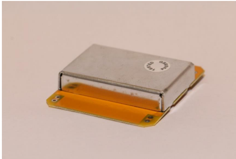
Figure 4-7 HB100 MC420S microwave module 10.525GHz with metal cover
