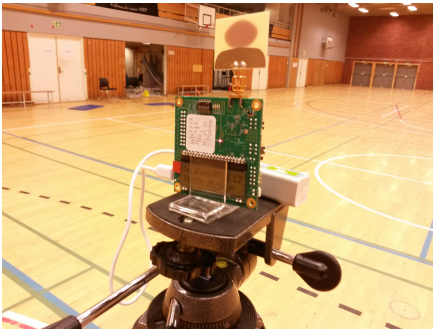
(c) The tag node was positioned on a tripod at one end of the gym hall and its position stayed constant throughout the experiment.
