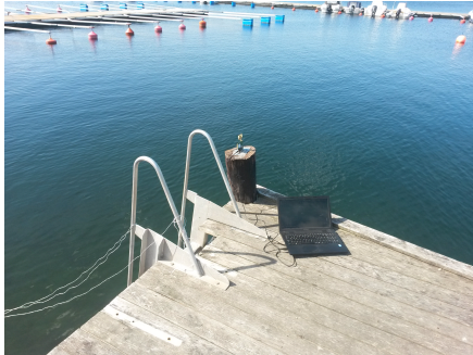
(c) Because of the limited resources available when the tests were carried out, and there was no extra tripod available, one of the anchors was positioned on a pole to give the sensor some height.
