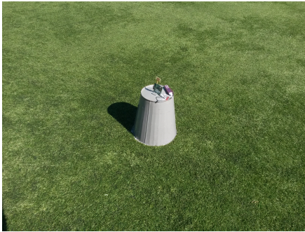
(c) The tag node was placed on top of an aluminum bucket to avoid placing it directly on the field.
