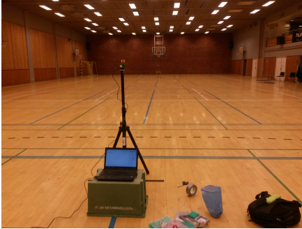
(a) The anchors were mounted on a tripod and connected to a computer to extract the measurements.
