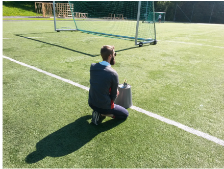
(d) A human blocked the tag node to see how well the sensors would perform in conditions with no line of sight.
