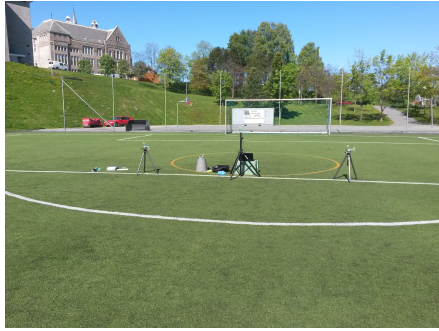
(b) Example of the closest setup of the anchors. The anchors were placed at a greater distance as well.
