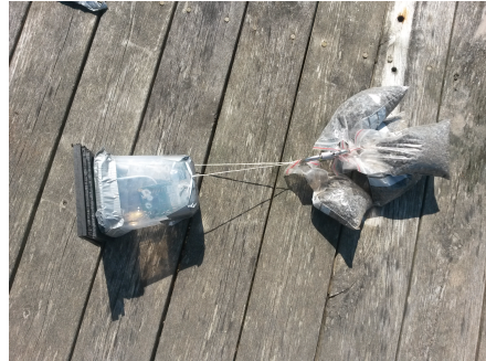
(d) The tag was put in a plastic box. Because the box was filled with air, bags with sand were used to get the desired buoyancy.
