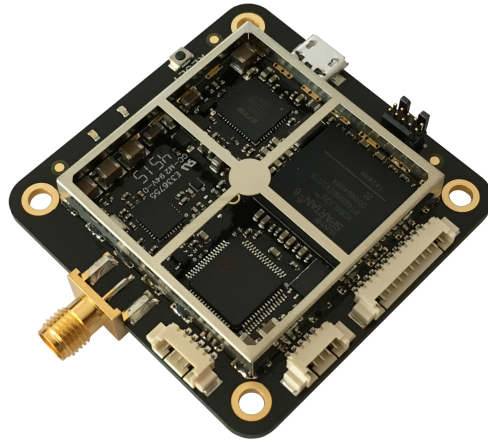
Figure 2.3: The Piksi GPS module was tested in an earlier phase of the project, but due to unsatisfying results an alternative approach is desired. Piksi™- Courtesy of Swift Navigation, Inc. | www.swiftnav.com
