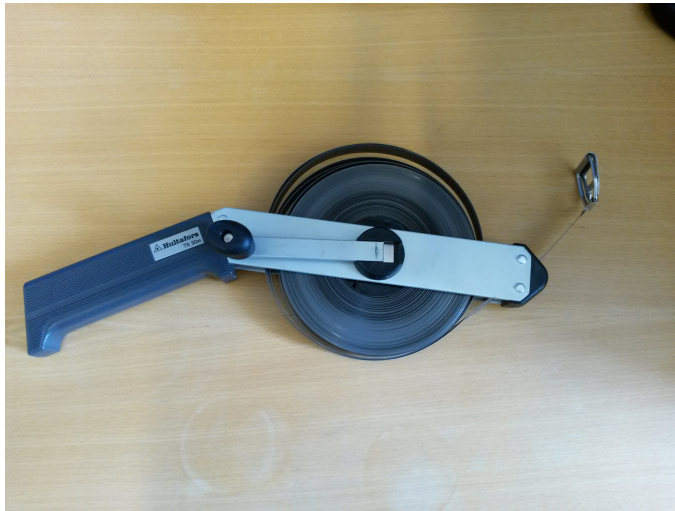
Figure 8.3: The tape measure used to measure the reference distances in the tests.
