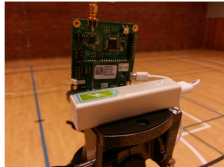
(d) Example of a power bank that was used as power supply for the circuit boards.
