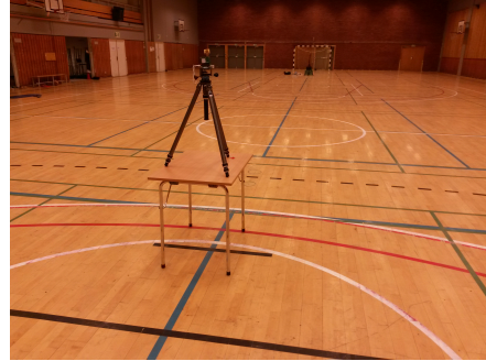
(b) Because of the height difference of the two tripods used in this experiment, one of the tripods had to be positioned on top of a table to make their height level.
