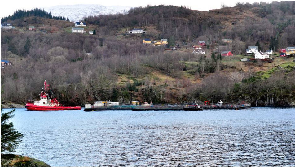
Figure 1.7: A tugboat in the process of saving an aquaculture installation from the pebble after the storm "Nina" caused failure in the mooring lines, leading the rig adrift in January 2015. (Gunn Berit Wiik Berg, Avisen Strilen)
