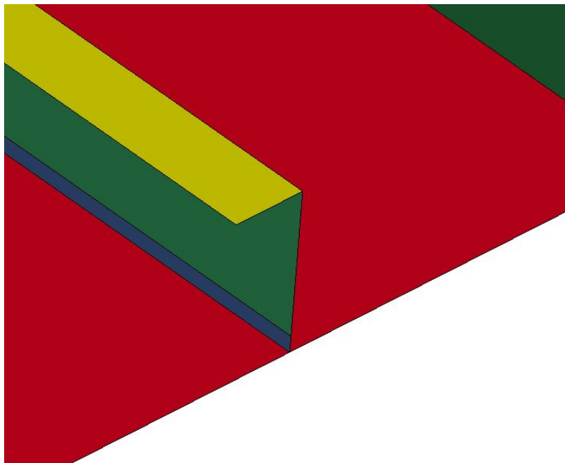
Figure 5.12: The Figure shows the modelling of stiffeners in the local model, the blue region is equal to 20\text{mm} height and represent the HAZ region
