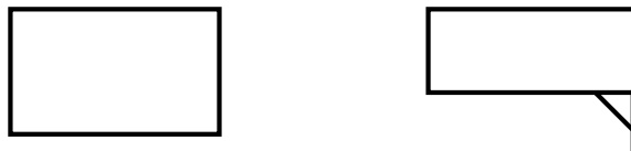
Figure 4.1: Cross section of the barrier, one closed symmetrical cross section and one cross section with skirt
