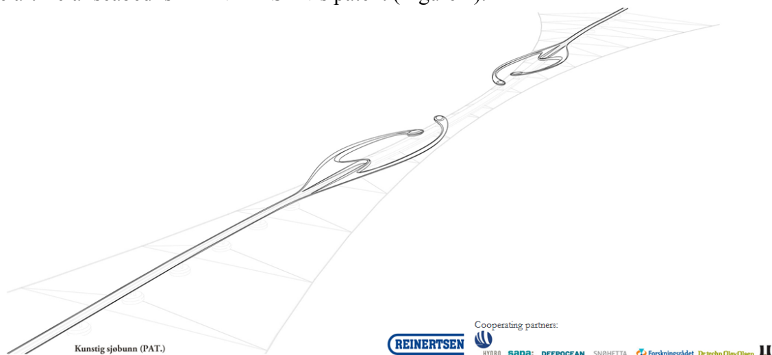
Figure 1 Concept with artificial seabed and mooring, floating bridge, submerged floating tunnel and collision barrier
