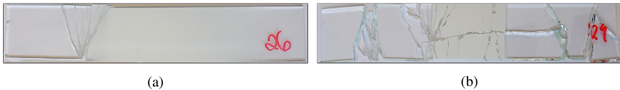
Figure 3: Typical glass specimens after failure in four-point bending tests: (a) failure at the edge, (b) failure at the face.
