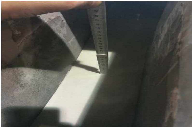
Figure 4.28: Picture of alumina level measurement
