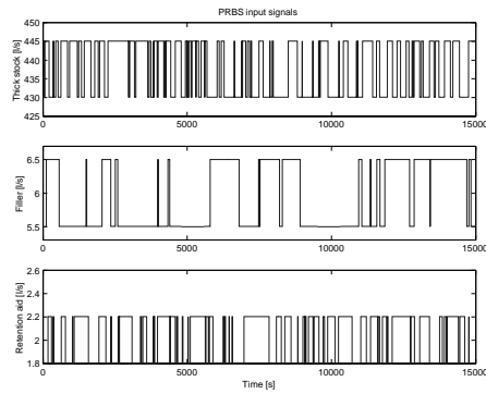
Figure 3: The filtered PRBS signals used for validation of the models. The overall operating condition of the paper machine is different from what was used for model identification and reduction.
