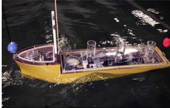
Figure 2.3: Cybership II with markers for positioning.
