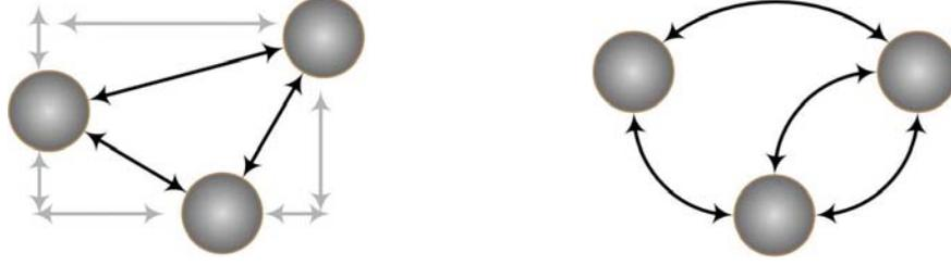
Figure 4.6: Examples of redundant auxiliary constraints. Consider the position offset constraints (4.21) on the left: when two constraints are given, the third is simply a linear combination of those. For the position relative constraints (4.20) on the right two of the constraints are either contradictory or redundant. In both cases, the Jacobian  $W$  has less than full row rank.
