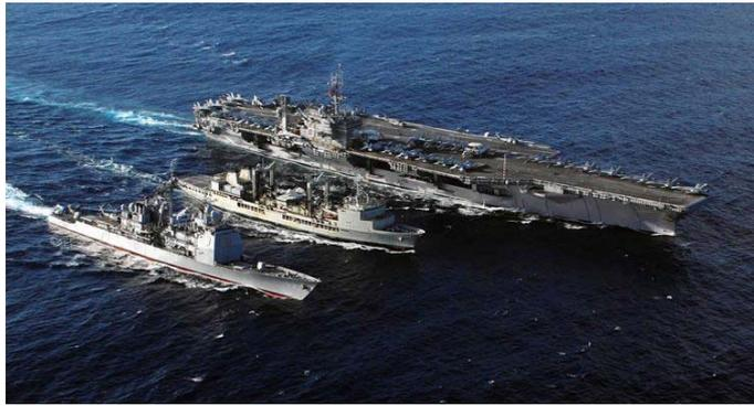
Figure 1.4: Double underway replenishment. Courtesy of U.S. Navy, [www.navy.mil](http://www.navy.mil).
