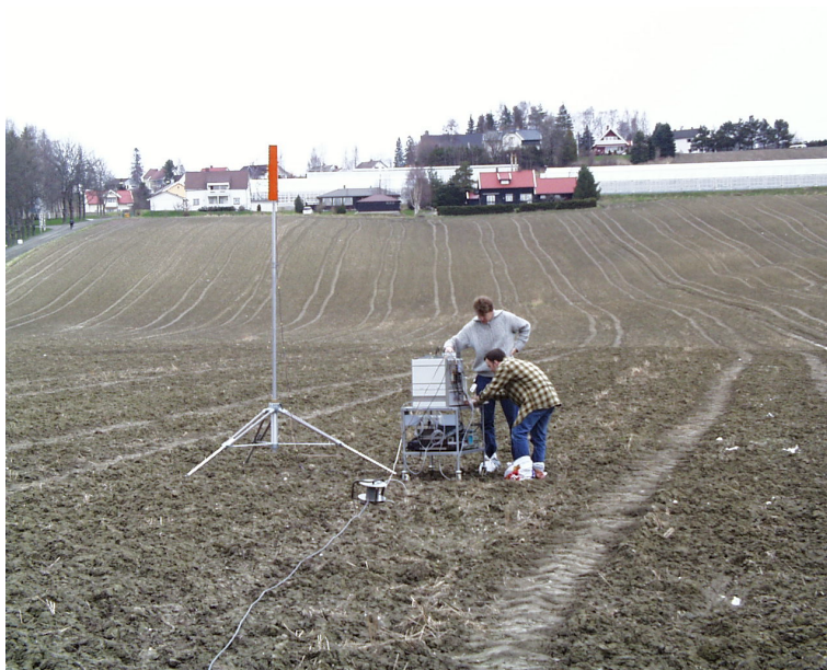
Figure 30. Picture of the grazing measurement set-up receiving side, the antenna array can be seen on the left
