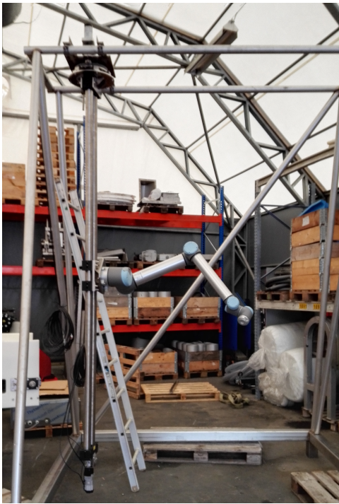
Fig. 5. The finished prototype. The lance and the spraying nozzle is not mounted.
