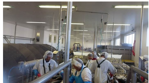
Fig. 2. The difficulties related to hoses, cables and pipes coming down from the ceiling further emphasised.
