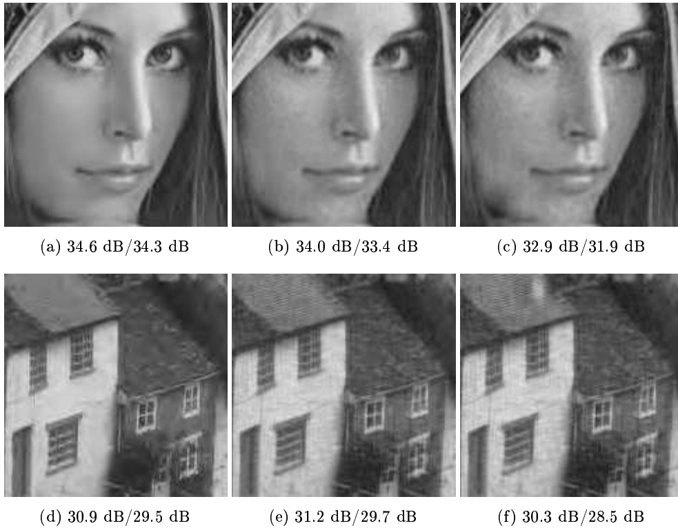
Figure 4.23 Extracts from “Lena” and “Goldhill” with a design CSNR of 20 dB and a total rate of 0.1 channel symbols per pixel. The left column shows the JPEG 2000 coding result, the middle column shows the result with the proposed coder at the design CSNR, and the right column shows the proposed coder at a CSNR of 17 dB. Under each extract, the PSNR of the whole image (with the applied noise sequence) and the PSNR of the shown segment are stated.
