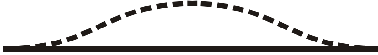
Figure 6.20: The solid line symbolizes the undeformed main beam. The dotted line shows the lowest eigenfrequency mode, which is used in the 2-d.o.f. model.
