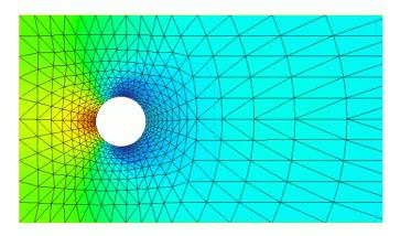
Figure 9.15 Flow around cylinder grid
