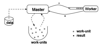
Figure 6.10 Pipelining of worker tasks
