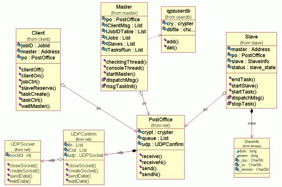
Figure 7.8 Simplified UML Diagram of QADPZ's architecture
