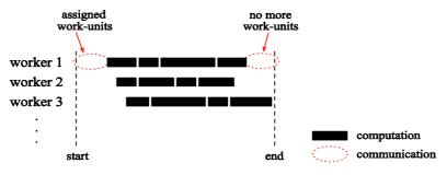
Figure 6.5 Computation times on workers: static decomp-static distrib
