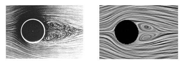
Figure 9.16 Flow around cylinder (measurement and simulation)
