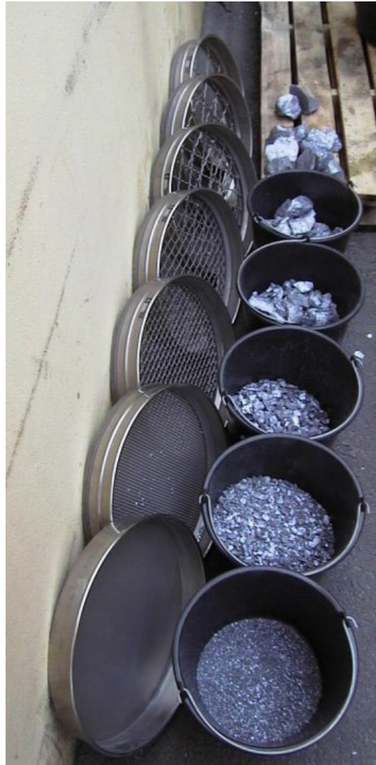
Figure 4.12: Sieve results of the FeSi feedstock.
