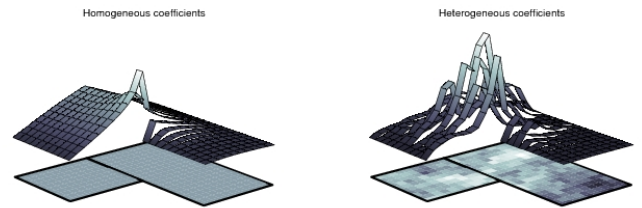
Fig. 2 - The x-component of the velocity basis function associated with an edge/face between two blocks of different size for a homogeneous and a heterogeneous permeability field, respectively.
