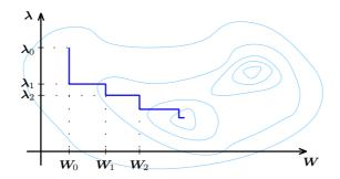
Figure 2.3: The coordinate descent method used to find the pair  $(\boldsymbol{W}^*, \boldsymbol{\lambda}^*)$  that minimizes the criterion function  $\mathcal{P}^{\log}_{\delta}(\boldsymbol{W}, \boldsymbol{\lambda}; \mathcal{D})$ .
