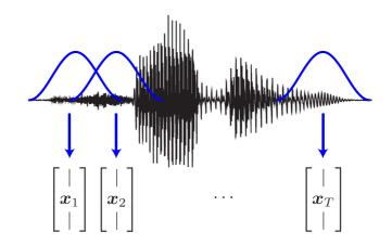
Figure 3.1: Feature extraction from a speech signal.
