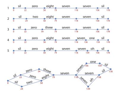
Figure 3.4: Top: An example of a 5-best list. The numbers under the nodes are frame numbers (in tens of milliseconds). Bottom: The lattice generated from the 5-best list above.
