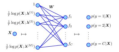
Figure 4.1: The logistic regression model with the likelihood mapping.
