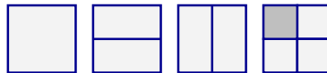
Figure 2.6 — Possible block splits of 16 \times 16 - and 8 \times 8 -pixel blocks. The gray-shaded block is thus either of size 8 \times 8 or 4 \times 4 pixels
