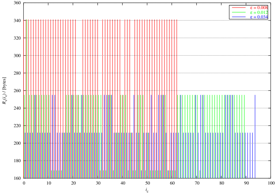
Figure 3.30 — Channel code distribution for the fourth GOP of QCIF -size Silent , coded with quality set B, as a function of the channel packet index under different channel conditions, i.e. with \epsilon as a parameter. The total number of channel packets necessary to transmit this particular GOP is equal to the maximum index value. The graph is continued in Fig. 3.31
