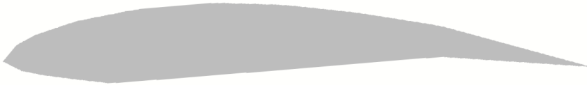
Figure 5.4: The NREL S826 airfoil represented by the .stl file from the turbine CAD model.
