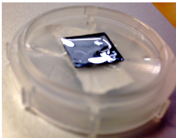
Figure 4.37: Photograph showing an example of an uncured sample, liquid phase deposited in pure FOTS solution. The photograph is recorded approximately 2 months after the sample was taken out of the immersion solution.
