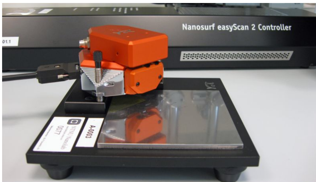
Figure 3.13: Nanosurf easyscan 2 Flex AFM used to obtain 3D-images displaying the roughness of the coatings.
