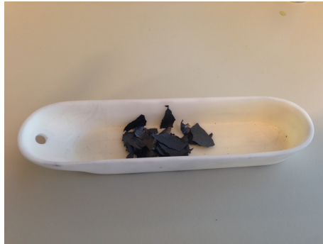
Figure 3.2: GO placed in an alumina boat before inserting it into the tube furnace.
