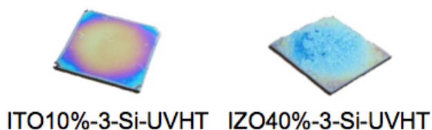
Figure 4.13: The UVHT cured thin films synthesized by deposition of ITO10%, and IZO40% solutions nr 3 on silicon substrates.
