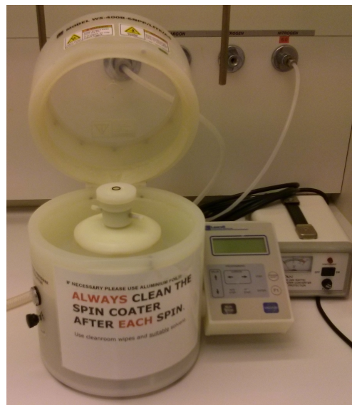
Figure 3.3: Picture of the Laurell Technologies, WS-400B-6NPP-LITE/ AS spin coater utilized.
