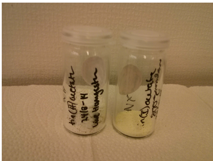
Figure C.16: Photograph of the new tin (II) acetate precursor. The untreated tin (II) acetate is to the left, while the tin (II) acetate heat treated at 800 °C in a calcination furnace is seen to the right.
