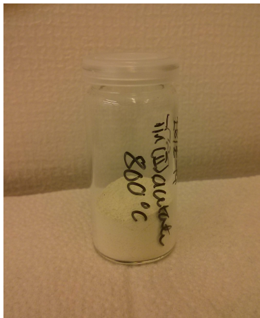
Figure C.12: Photograph showing the resulting powder after heating the tin (II) acetate precursor to 800 °C in a calcination furnace.
