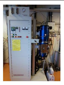
Figure 4.1: The Resina furnace
