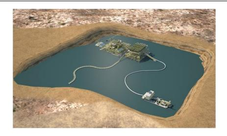
Figure 2.2: Graphical representation of dredging operation (courtesy Tizir, Norway)
