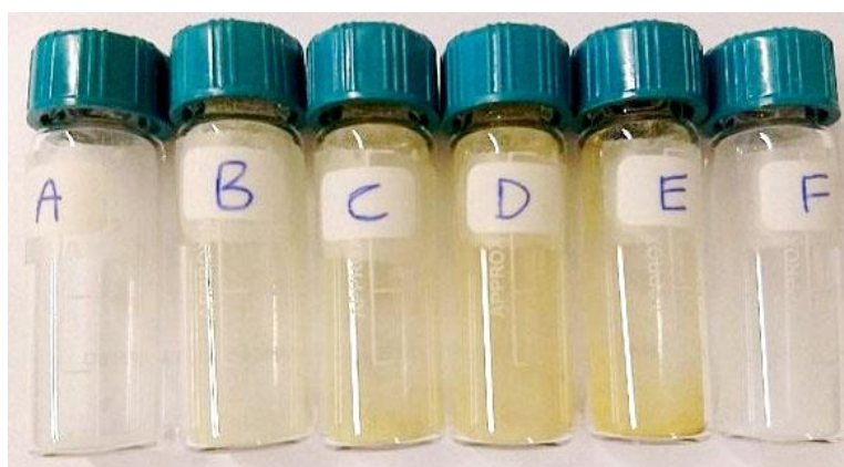
Figure 4.10: Image PS-10 photodegraded for (A) 0, (B) 10, (C) 20, (D) 40 and (E) 80 days and (F) control sample ( t_{40} ) not irradiated but otherwise weathered under the same conditions for 40 days.
