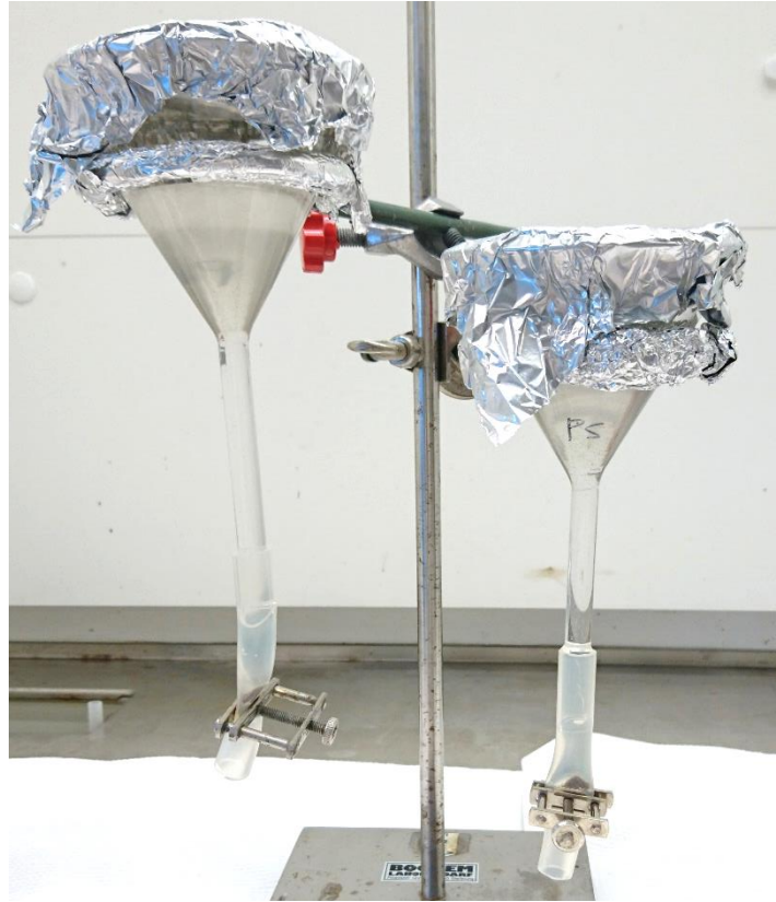
Figure 3.3: The set-up of the density separation, to separate microplastic particles from soil.
