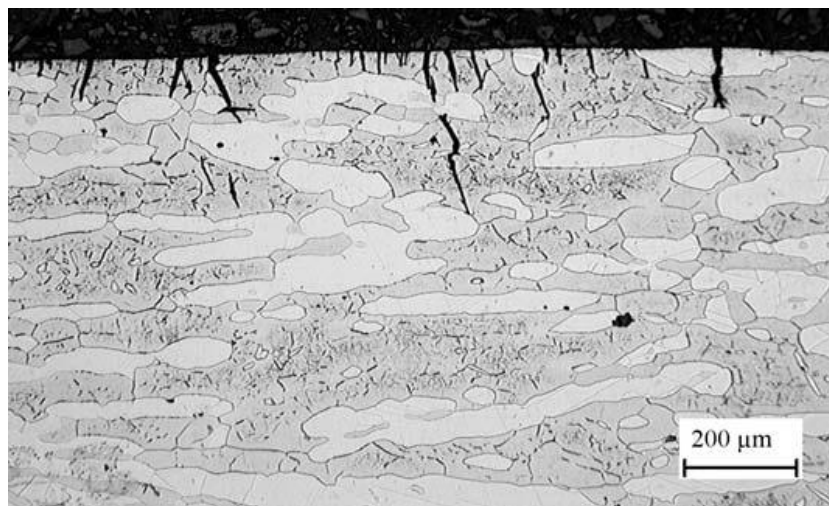
Figure 12 Shallow cracks in a SDSS. [1]
