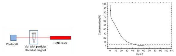
**Figure 6.** Left: Experimental setup to measure how fast 50 nm beads with a 40 nm iron oxide nanoparticle core can be separated with GIAMAG. The vial was a 2 ml microcentrifuge tube strapped to the surface of the magnet. The amount of light from the laser beam detected by the photocell is a measure of the remaining dispersed particle concentration. Right: The measured concentration of the nanoparticles still in the solution versus time.
