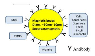
**Figure 2.** Schematic the wide use of magnetic bioseparation. The magnetic micro- and nanoparticles need to be functionalized, i.e. treated with appropriate surface coatings, like antibodies, to be able to target various biosystems as discussed in the text.
