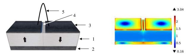
Figure 4. Left: Schematic outline of the original design of the GIAMAG magnet. The system consists of the following key components: Two adjacent permanent magnets (1) with opposite direction of magnetization, a yoke (2) and masks (3). The design involves a small gap (4) producing a very strong magnetic field gradient (5). Right: Computer simulation of the magnetic field strength distribution on the surface with N52 grade Neodymium–iron–boron magnets. The color scale is given in Tesla.
