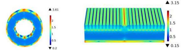
**Figure 5**. Left: A cylindrical GIAMAG magnet design where 8 gaps run axially. The yoke is placed on the outside and the masks on the inside. The color scale is given in Tesla. Right: A GIAMAG magnet design with many separate masks. The color scale is given in Tesla.
