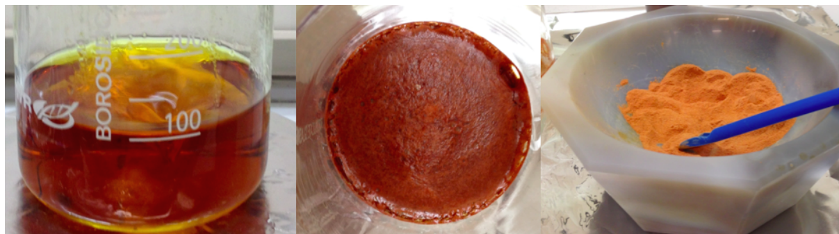
Figure 3.7: An illustration of the different stages in the process of obtaining a raw powder of \text{YbFe}_2\text{O}_4 from sol-gel synthesis .
