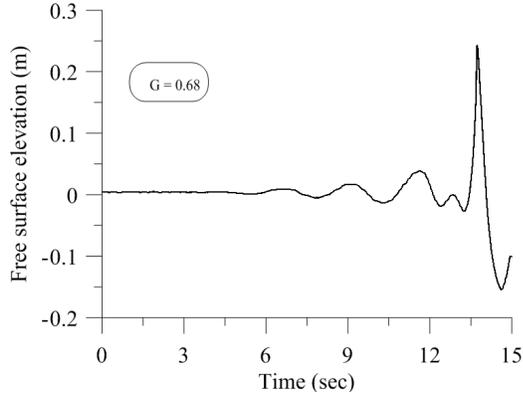
Fig. 5b. Free surface elevation at focus point for P2
