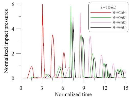
Fig. 8. Comparison of normalized pressures at SWL ( $Z/H_b = 0$ ) for four different plunging cases
