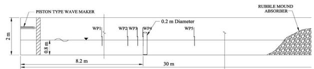
Fig. 2. Sectional view of experimental setup for cylinder with horizontal sea bed
