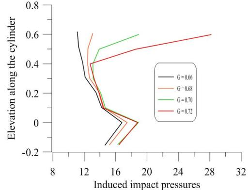
Fig. 10. Variation of induced impact pressure along the elevation of cylinder for four different plunging cases
