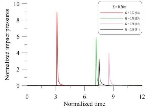
Fig. 7. Comparison of normalized pressures at  $Z = 0.26\text{m}$  ( $Z/H_b = 0.64$ ) from SWL for four different plunging cases
