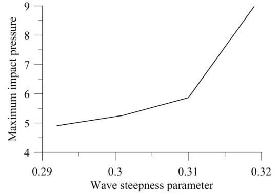
Fig. 11. Variation of maximum impact pressure for four different wave steepness parameters
