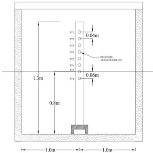
Fig. 3. Sectional view of cylinder with pressure transducers
