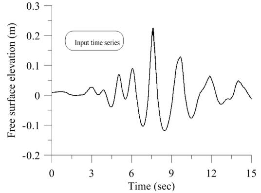
Fig. 4. Input time series to wave maker for constant steepness wave packet
