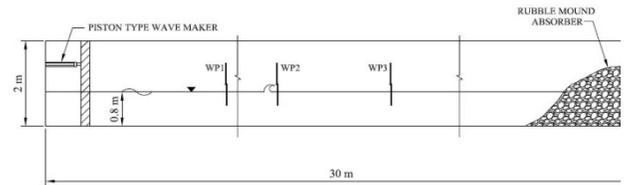
Fig. 1. Sectional view of wave flume with wave probes
