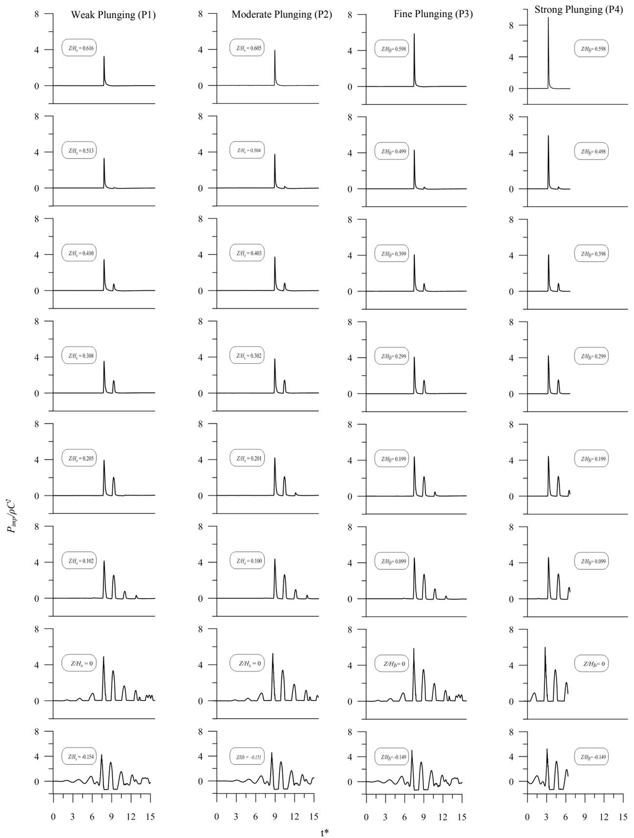
Fig. 6. Temporal variation of normalized pressure time history at elevations along the front case of the cylinder for four different plunging cases
