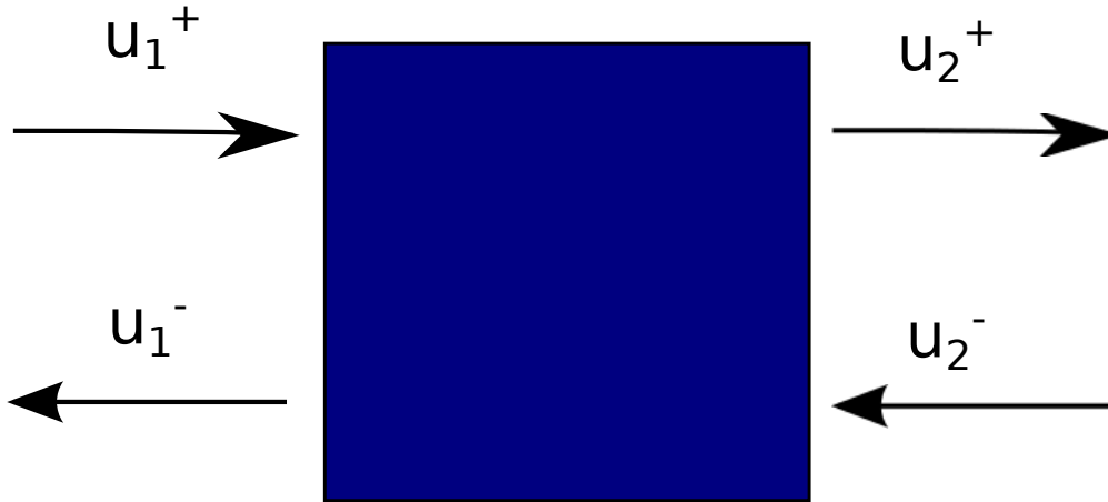
Figure 2.2: One period of the photonic crystal. u_1^+ is the incoming wave to the left, u_1^- is the outgoing wave to the left, u_2^+ is the outgoing wave to the right and u_2^- is the incoming wave to the right.
